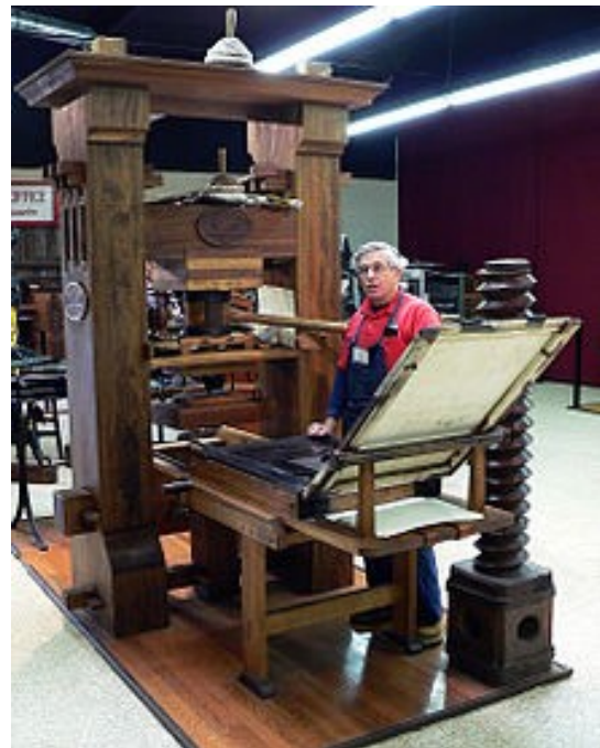
A rebuilt copy of the printing press invented by the gold smith Johannes Gutenberg in 1440. It had a capacity of 3600 pages a day
